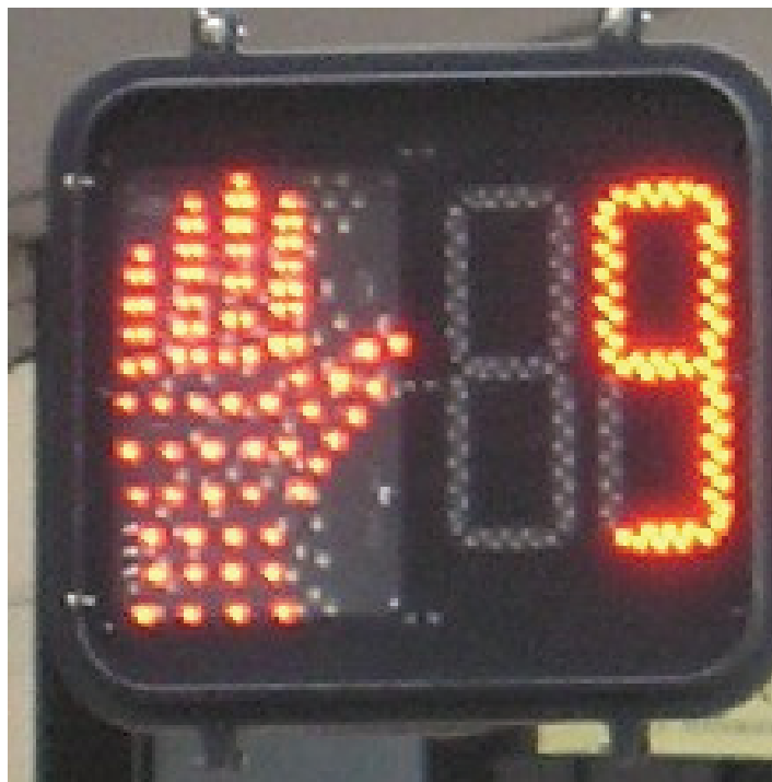
Countdown pedestrian signals convey the actual time a pedestrian has to safely make it through an intersection
